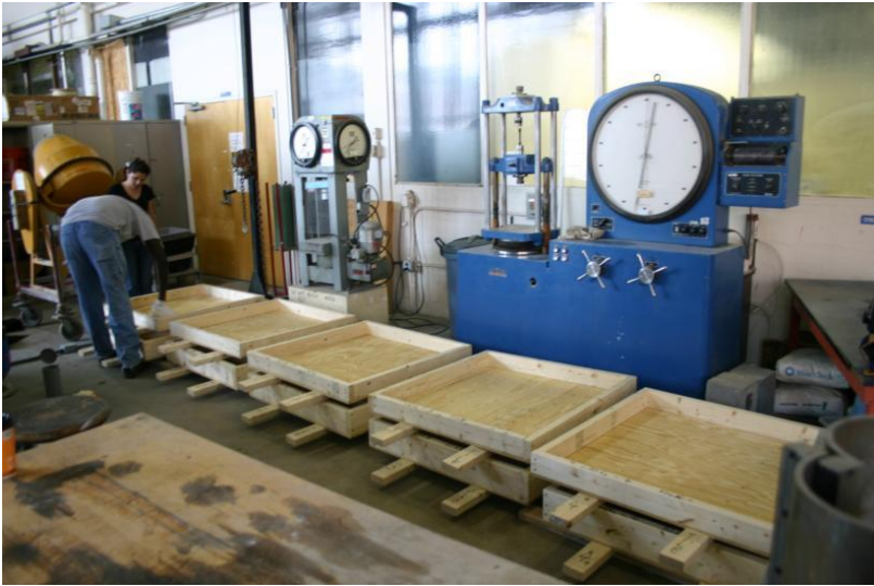
Figure 5-6- Specimens' form work
